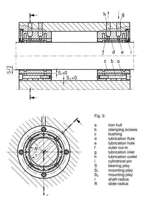
The inner bushing has some axial lubrication flutes (d) which are connected with the outer cut-in (f) in the steel hull by radial lubrication holes (e). By this arrangement the bushing is connected with the lubrication inlet (g) and outlet (h) in the housing bore.
