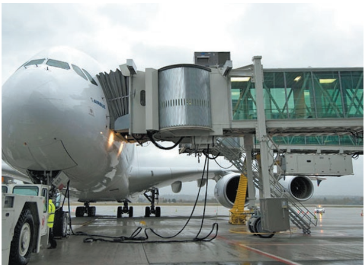
FMC Jetway Apron Drive Passenger Boarding Bridge. © 2007 Photo by P. Michaud. Courtesy of FMC Technologies, Jetway.
