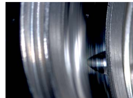
Ball indentation in raceway
